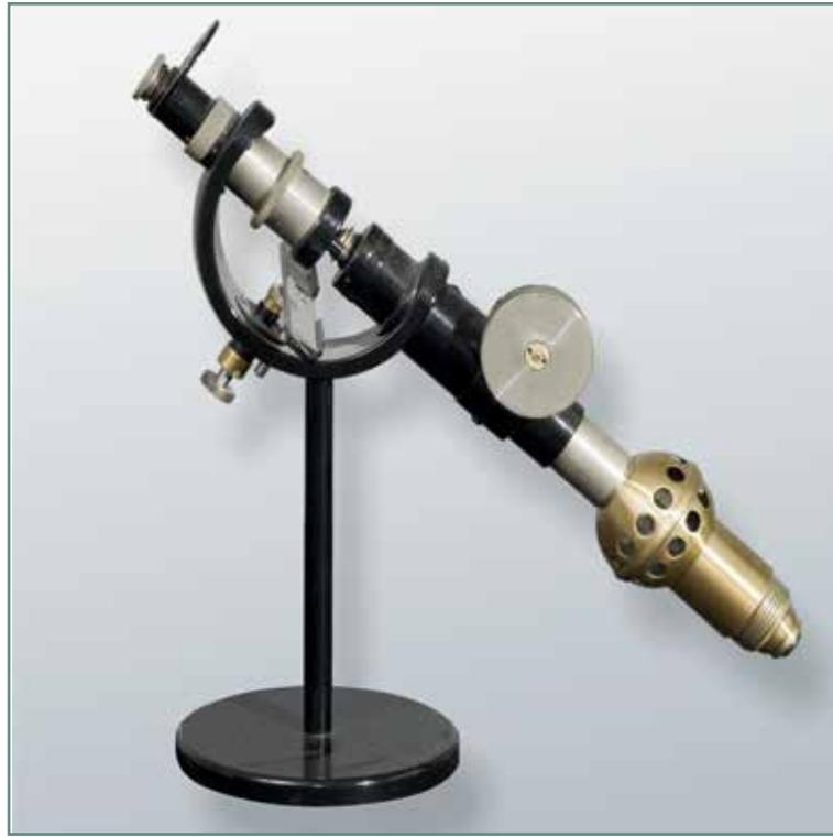
Focimeters allow accurate determination of the spherical and cylindrical power of lenses and also indicate the axis of the cylinder. The first fociometer or lensmeter was designed by Hermann Snellen in 1876 and was known as a phakometer (fig.1). It was constructed by Dirk B Kagenaar (1842-1927) in the laboratory of the Eye Hospital in Utrecht. It very much resembles an optical bench.
