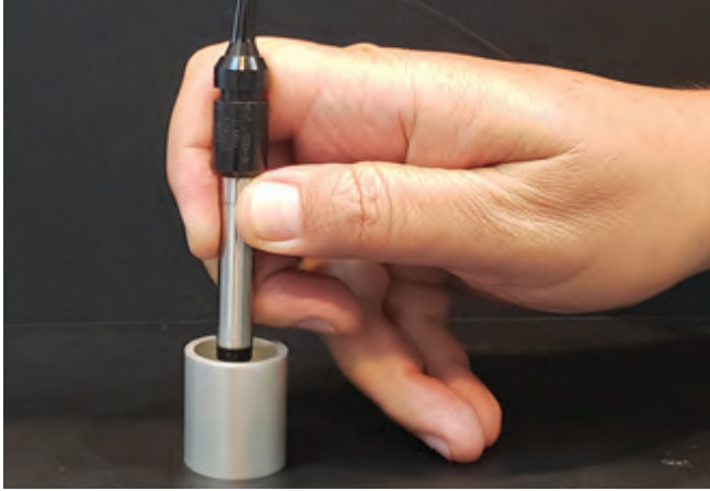
Fig 19.1: Calibration of the probe to using the tissue model (TM 868) in order to obtain tissue sensitivity.
