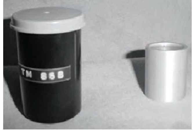
Fig 19.1: Calibration of the probe to using the tissue model (TM 868) in order to obtain tissue sensitivity.
