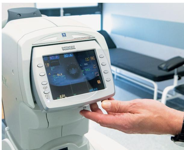
Figure 3. Non-contact “air puff” tonometer.
