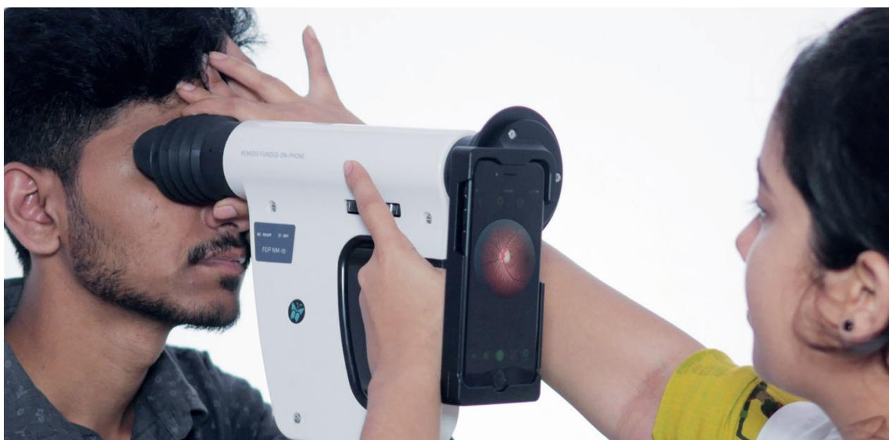
Figure 3. The Fundus on Phone ophthalmoscope attachment produced by the Indian company Remidio.
